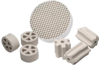
All inert top gradings are developed to replace inert ceramic balls and alumina balls at the top of catalytic reactors, by increasing distribution properties and void fractions to extend cycle length of the units. The larger void fraction and different shapes allow better resistance against particulate deposition (solids such as rust, gum, coke, etc.) or top bed crust formation.
